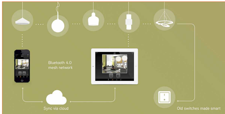
Figure 2: A typical Bluetooth 4.0 lighting mesh network configuration
