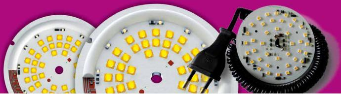
This new technology replaces conventional powersupplies by working with out capacitors, inductors, transformers and all components, which have limited lifetime. By newest IC technology the complete drivers can be placed on a LED module for direct connection to 230 VAC.
