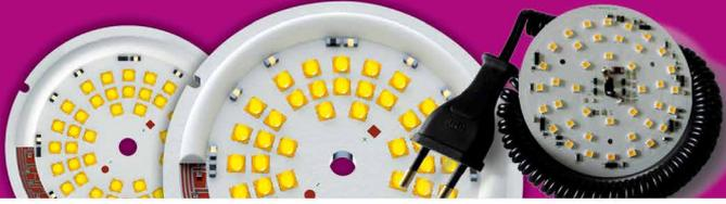
This new technology replaces conventional powersupplies by working with out capacitors, inductures, transformers and all components, which have limited lifetime. By newest IC technology the complete drivers can be placed on a LED module for direct connection to 230 VAC.
