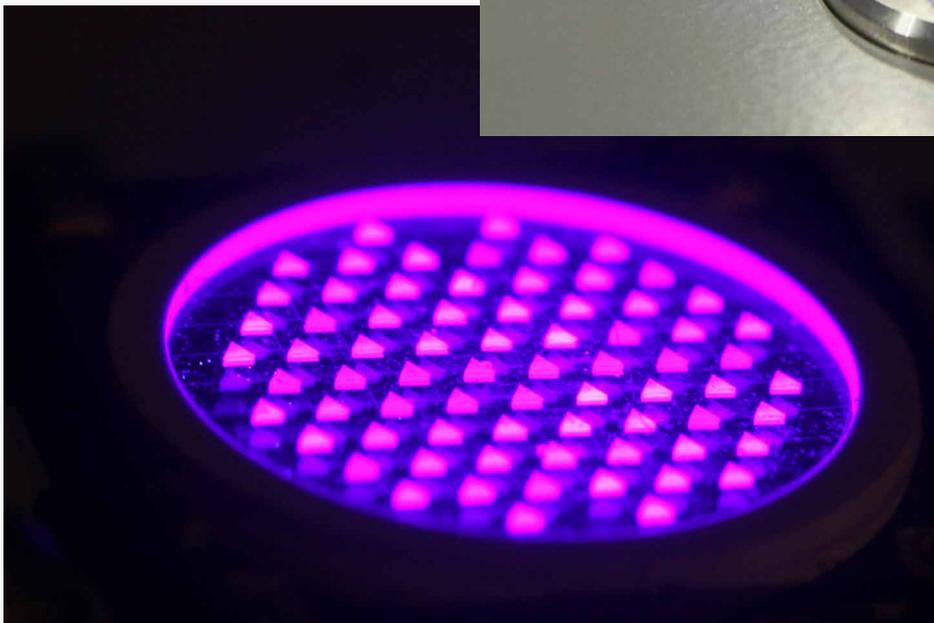
◀ **Soraa** brought an array of LED samples that showcased their unique triangular dies. The crystal lattice structure of GaN-on-GaN wafers makes it possible to cut triangular dies. The advantage of this geometry is that, compared to squares, extraction losses are reduced.
