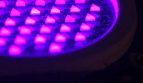
► **Soraa** brought an array of LED samples that showcased their unique triangular dies. The crystal lattice structure of GaN-on-GaN wafers makes it possible to cut triangular dies. The advantage of this geometry is that, compared to squares, extraction losses are reduced.
