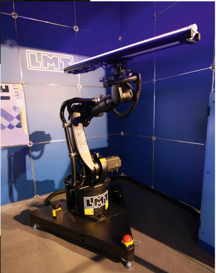
► **LMT Lichtmesstechnik GmbH Berlin**, a renowned light measurement specialist, introduced their brand new KUKA robot based goniometer. While the use of KUKA robots for measurement tasks is not new, LMT made significant changes and improvements to the software to better accommodate light measurement tasks.
