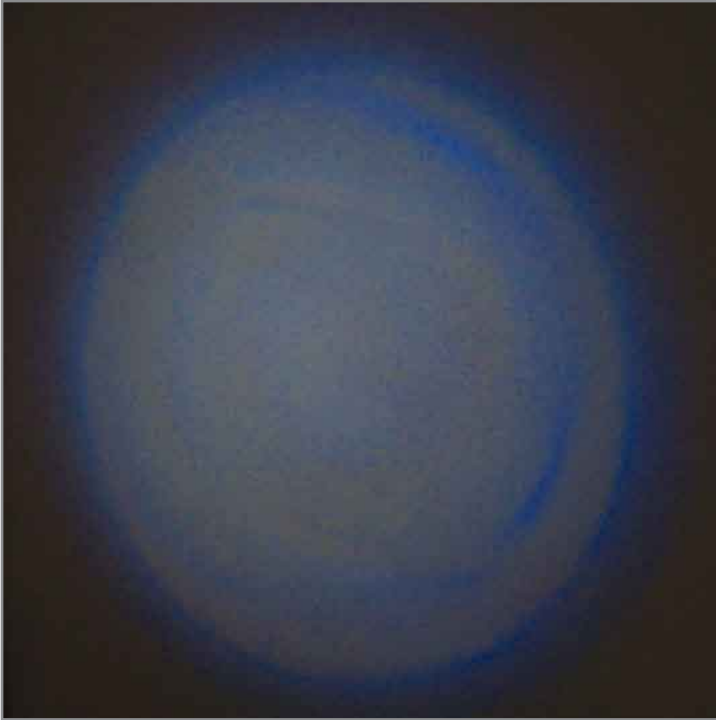
Figure 8: Beam pattern of LED spotlight with bluish and yellowish regions resulting from different light path length through phosphor
