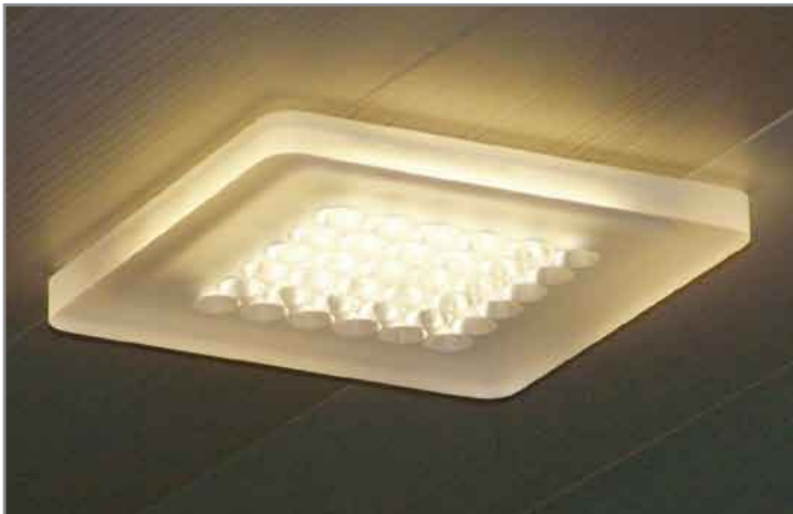
Figure 4: LED downlight - 36 LED (3000 K) with total power consumption of 9 W and light output of 470 lm replaces incandescent lamp with 40 W.
