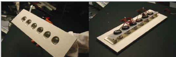
The low profile LED fittings were designed to fit into a cavity just 5 cm deep while keeping the LEDs satisfactorily cool.
