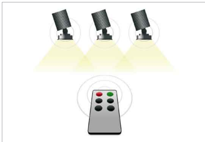
Figure 6: Wireless dimming using a remote control.
