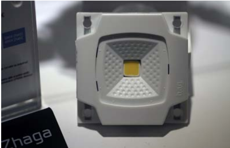
Figure 5: Zhaga Book 7 compliant LED modules were already presented at Light+Building 2012 in Frankfurt
