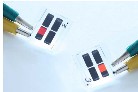
Liquid-processed SiLEDs: By changing the size of the silicon nanocrystals the color of the emitted light can be varied (Photo: F. Maier-Flaig, KIT/LTI)
