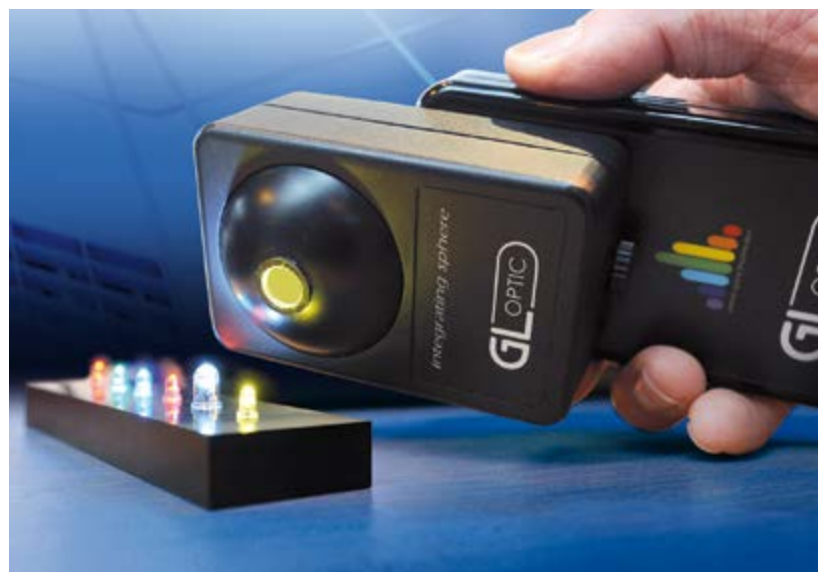
Figure 3: Small integrating spheres are also used in high quality handheld instruments for single LED measurements
