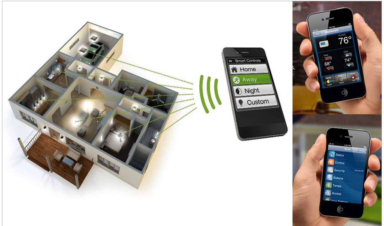
Figure 4: Different interfaces are available to control BAS. Apps for lighting controls, HVAC and many other tasks are available for smart phones and tablets using Android or iOS
