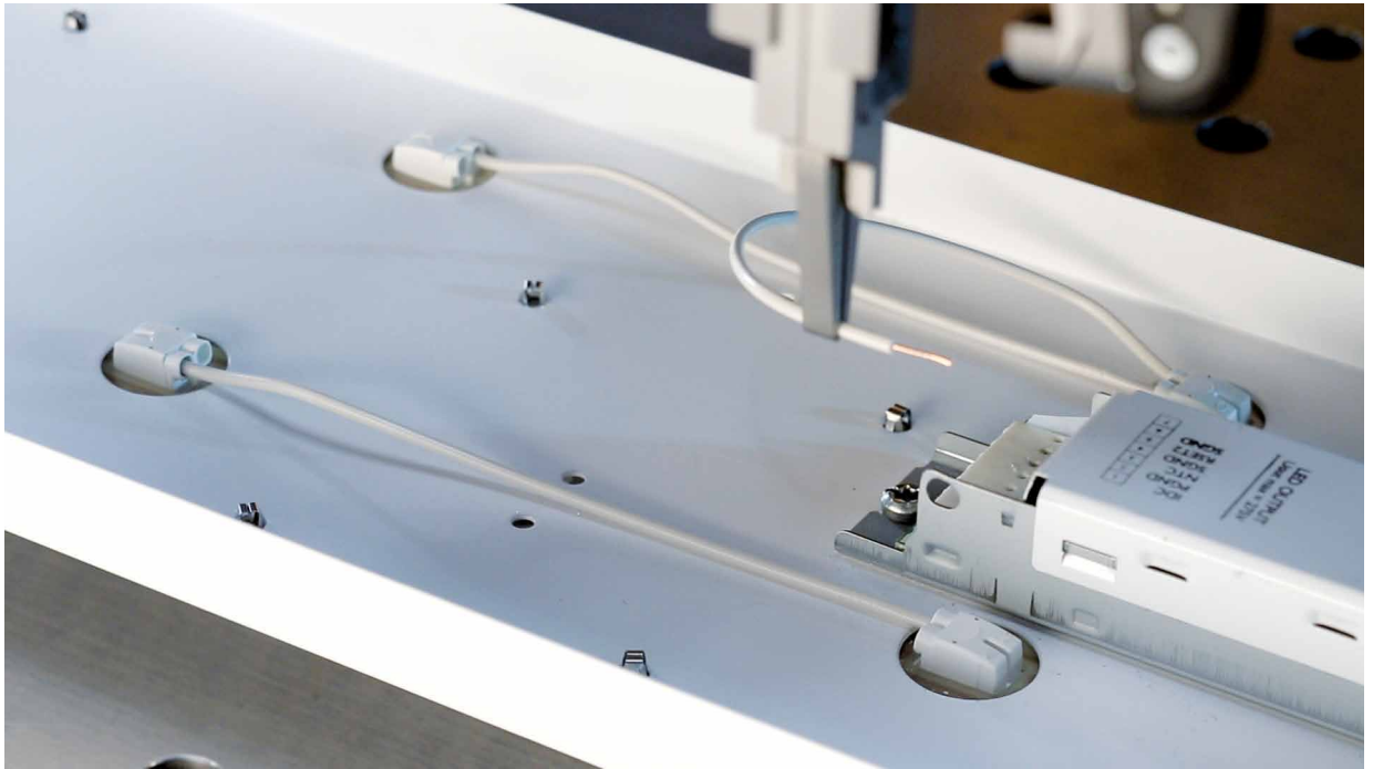
Figure 4: The SMD terminal block for rear-side wiring speeds up production of luminaires with control gear on the rear side of the mounting plate, as it is not necessary to turn the luminaire during assembly
