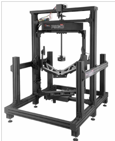
Figure 3: Goniophotometer used in this investigation
