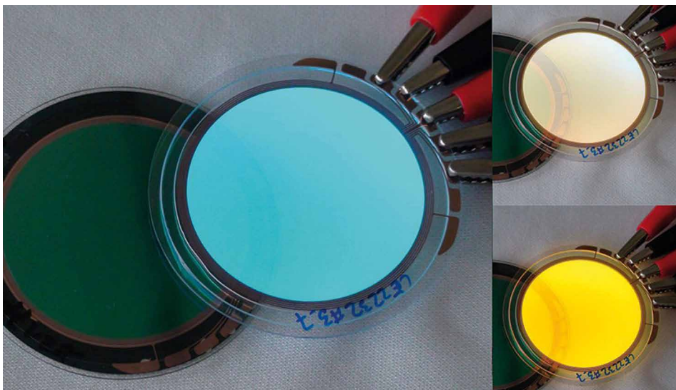
The color tunable OLED modules have a diameter of 55 mm with an active light area of 42 mm
