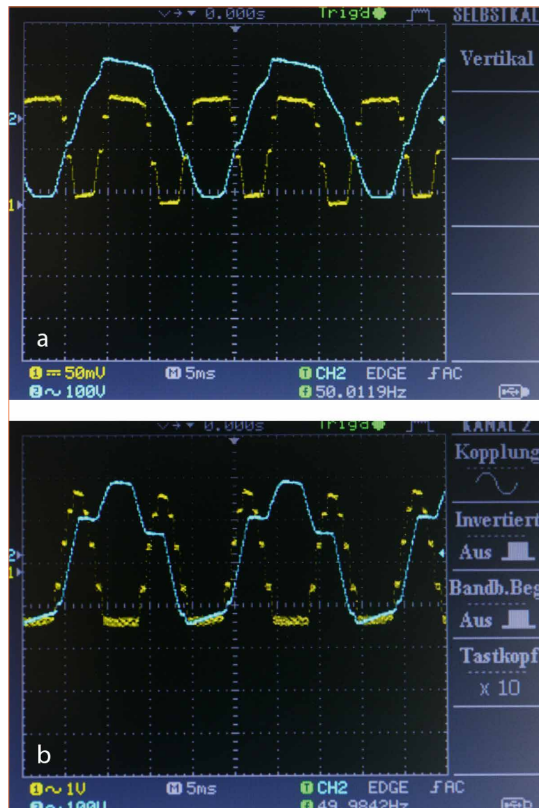
Figures 4 a&b: Light fluctuations of different AC driven LED modules. The new concept: trapezoidal light curve (a), LED module using a conventional concept: wedge-shaped light peaks (b) (luminous flux modulation is measured with an ultrafast photodiode in normal operation and dimmed)
