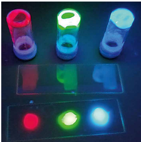
Gel-like networks consist of a concentrated aqueous protein solution and a polymer compound (Image: Michael Weber)
