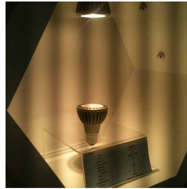
Figure 5: Flicker detection using the built in camera of a cell phone obtained by LAPLACE. Flicker leads to the appearance of dark fringes on the image
