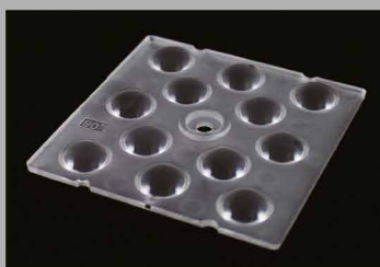
LL12ZZ-CRC90L19 DxWxH(mm) 50x50x3.8 FWHM 90° Edison 3030 Lumileds Luxeon 3030 Nichia 757D
