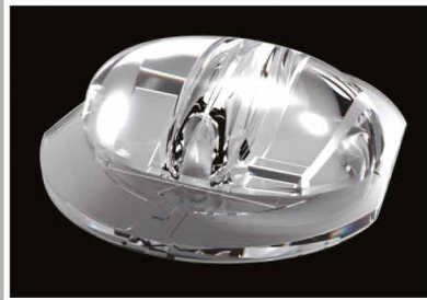
LL01CR-CQW60155L100 DxWxH(mm) 99.7x110.5x30.98 FWHM 60x155° Cree CXA3050 Citizen CLL040/042 Lumileds L2C1-1211
