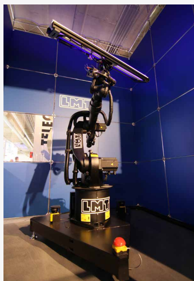
LMT Lichtmesstechnik GmbH's latest KUKA robot based goniometer
