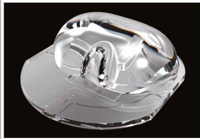
LL01CR-CQW45150L100 DxWxH(mm) 99.7x110.5x32.78 FWHM 45x150° Cree CXA3050 Citizen CLL040/042 Lumileds L2C1-1211
