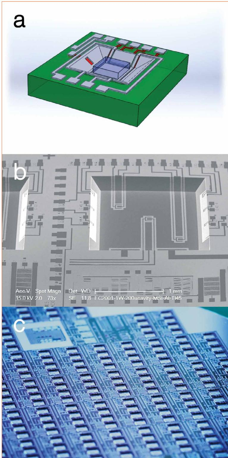
with a 200  $\mu\text{m}$  KOH cavity coated later with a thin aluminum layer to form a mirroring sidewall. Furthermore, temperature and light sensors were fabricated on the cavity bottom and sidewall, respectively. The wires for LED driving current and sensor connections were patterned the whole way from top surface to cavity bottom. The fabrication process
