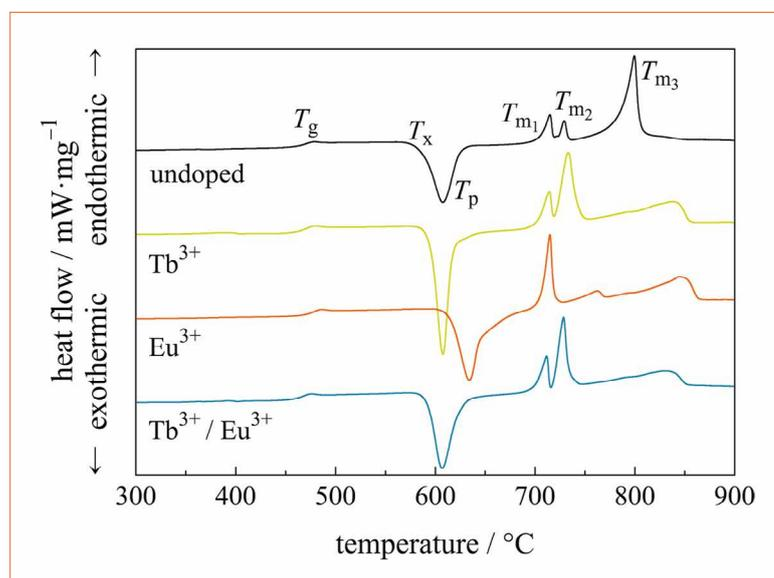
**Figure 2:** DSC data of the undoped reference glass (black), Tb<sup>3+</sup> doped (green), Eu<sup>3+</sup> doped (orange), and Tb<sup>3+</sup>/Eu<sup>3+</sup> double-doped borate glass (blue)
