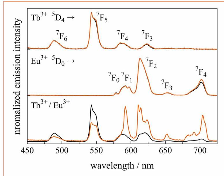
**Figure 4:** Emission spectra of glasses (black curve) and glass ceramics (orange curve) doped with  $\text{Tb}^{3+}$  (top),  $\text{Eu}^{3+}$  (middle), and  $\text{Tb}^{3+}/\text{Eu}^{3+}$  doped (bottom). All emission spectra are recorded under 376-nm excitation
