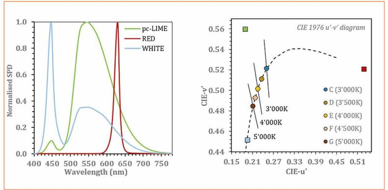
**Figure 8:** Calculated emission spectra (left) expected for 3,000K (C), 3,500K (D), 4,000K (E), 4,500K (F) and 5,000K (G) obtained with 3014L and 3535L red and pc-lime LEDs at different relative radiant flux levels. The CIE u'v' coordinates (right)
