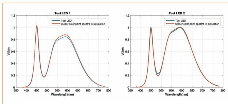
**Figures 4:** Two new LEDs, measured and compared with spectra in cloud above where the color point is as close as possible
