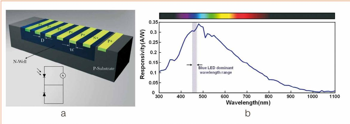
**Figure 5a,b:** 3D schematic of a blue selective photodiode (a), and responsivity vs. wavelength (b), measurement result (the patterned inset shows the dominant wavelength of the target LED)
