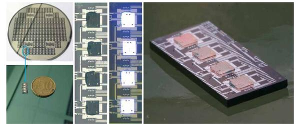
**Figure 4:** Monolithically integrated 2D LED SiP
