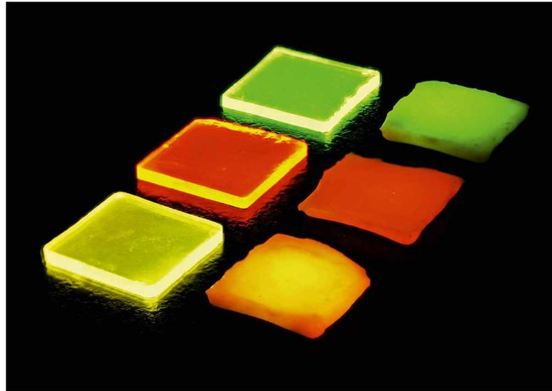
**Figure 1:** Ln<sup>3+</sup>-doped borate glasses (left) and glass ceramics (right): Tb<sup>3+</sup> doped (top), Eu<sup>3+</sup> doped (middle), and Tb<sup>3+</sup>/Eu<sup>3+</sup> double-doped (bottom) under ultraviolet irradiation
