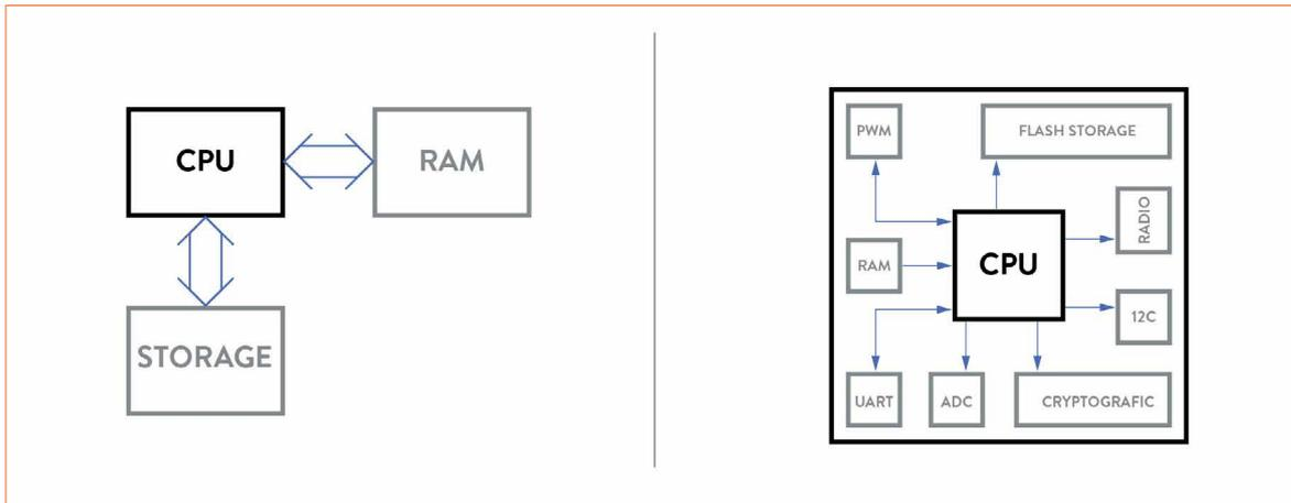
**Figure 1:** A traditional computer architecture can be seen on the left. All major components are separate chips interconnected via data magistrale. A typical SoC architecture is presented on the right. All SoC components are integrated into single chip and connected internally
