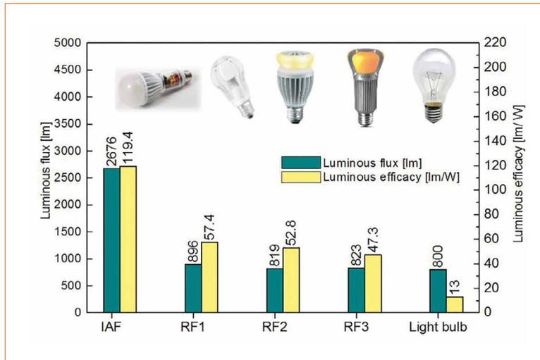
Spectral photometry measurements reveal that with the same lamp size a luminous flux of 2676 lm is achieved, which is three times higher than that of commercial retrofits, with an overall luminous efficacy of 119.4 lm/W (Figure 6).
