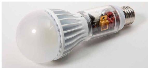
Figure 4: LED lamp in E27 bulb form factor with a power converter based on a GaN HFET in TO-220 package (section containing the power converter extended for demonstration purposes)
