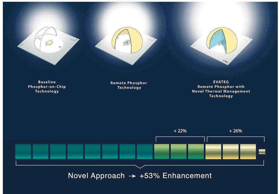
A combination of remote phosphor with an innovative thermal management approach adds 53% lumen extraction efficiency
