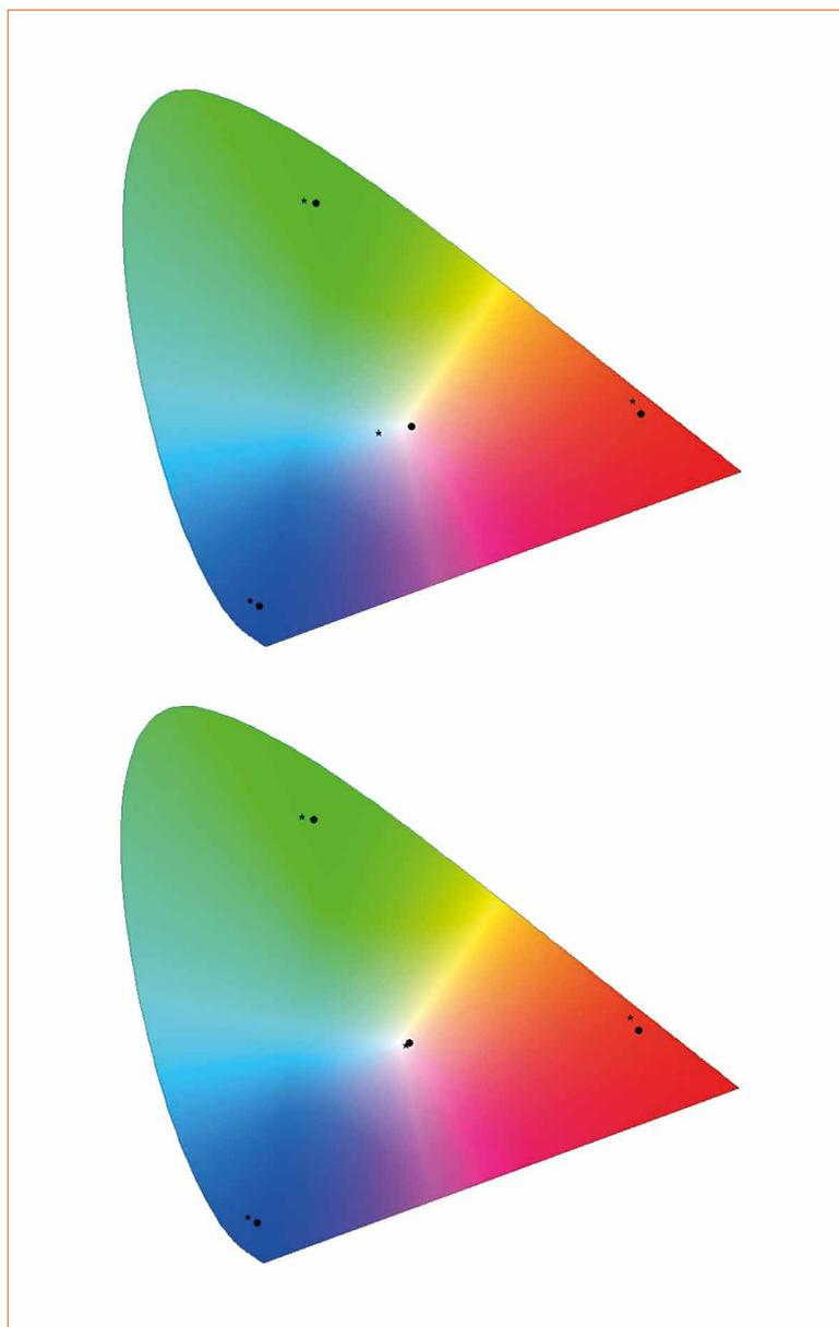
This method is a relatively straightforward way of balancing the colors between two different luminaires. This is a simple method of determining the compensation factors, especially when choosing the correct RGB bins to ensure the primary colors match. A disadvantage, however, is when applying this method to RGB LEDs from different bins. In that case, even with an identical white point the saturated colors can appear different.
