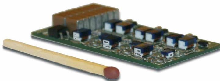
Figure 8: Electrolytic free 60 W LED driver
