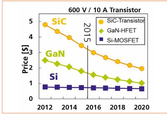
Figure 1: Expected average selling price of a single 600V/10A transistor based on Si, SiC and GaN [4]
