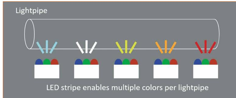
Figure 2: Color LED strip with individual color control
