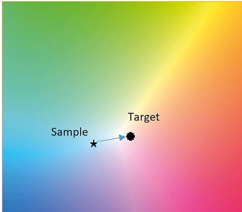
This calibration process provides a compensation factor for each individual LED inside the RGB LED.
