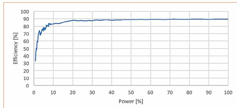
**Figure 5:** Efficiency curve for the 20 W driver operating at 30 MHz
