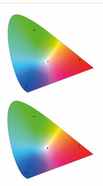
This calibration process provides a compensation factor for each individual LED inside the RGB LED.
