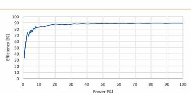
operating under optimal conditions with the highest efficiency or off with will low losses. This enables a very flat efficiency curve. This can either be used to achieve higher dimming efficiency in a specific luminaire or to use a given driver across a wider set of luminaires while achieving high efficiency for all.
