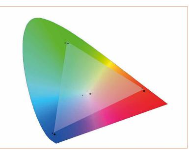
color points. The final result is an exact overlap of the gamut of the sample and target light source. With reference to Figure 5, a perfect color gamut match means the 'triangles' of both the target and sample light sources perfectly match one another. As with white point calibration, the method for gamut calibration is straightforward:
