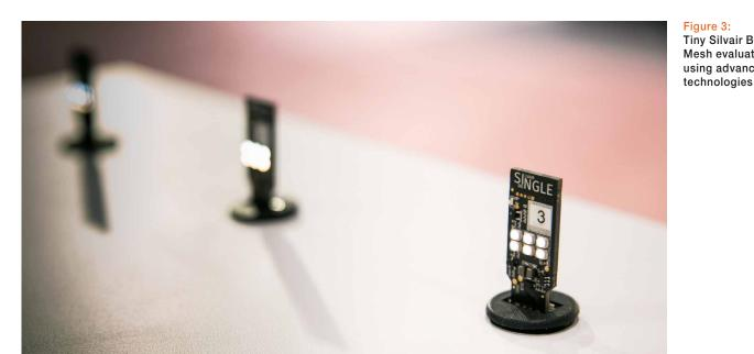
Figure 3: **Tiny Silvair Bluetooth** Mesh evaluation nodes using advanced SoC
