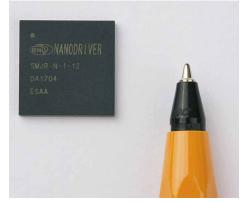
NanoDriver Series phase-cut LED drivers measure just 13.5mm x 13.5mm x 1.42mm
