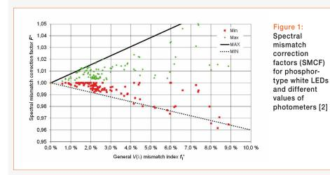
contribute a maximum of about 4.8% to the uncertainty when measuring phosphor-type white LEDs. In most cases this is the dominant uncertainty parameter in the measurement of LED lamps and luminaires when the measurements are performed using photometers. According to the international LED measurements standard (CIE S 025, [2]) the measurement uncertainty shall be reported as part of the measurement results.
