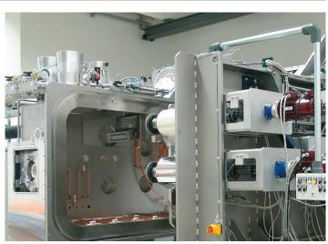
A roll-to-roll process is the key to affordable large area flexible OLEDs
