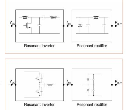
voltage, but for applications with high input voltage (such as mains), a voltage stress of 3.5 times the input voltage across the switch is a major drawback of this topology. If designed to operate in the optimum situation, the inductors are the largest for any of the topologies that limits the transient response and the power density. However, the inverter can be designed to operate in a sub nominal situation with smaller inductors and faster transient response.
