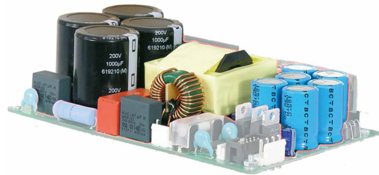
Figure 1: A traditional power supply where passives constitute most of the volume
