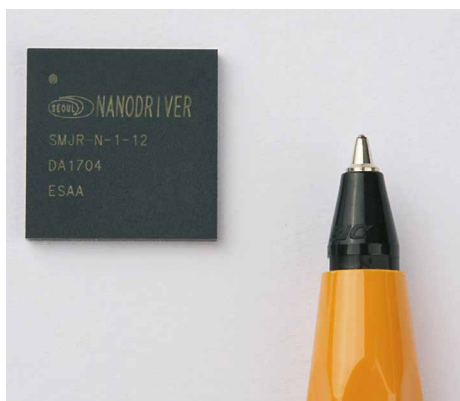
NanoDriver Series phase-cut LED drivers measure just 13.5mm x 13.5mm x 1.42mm
