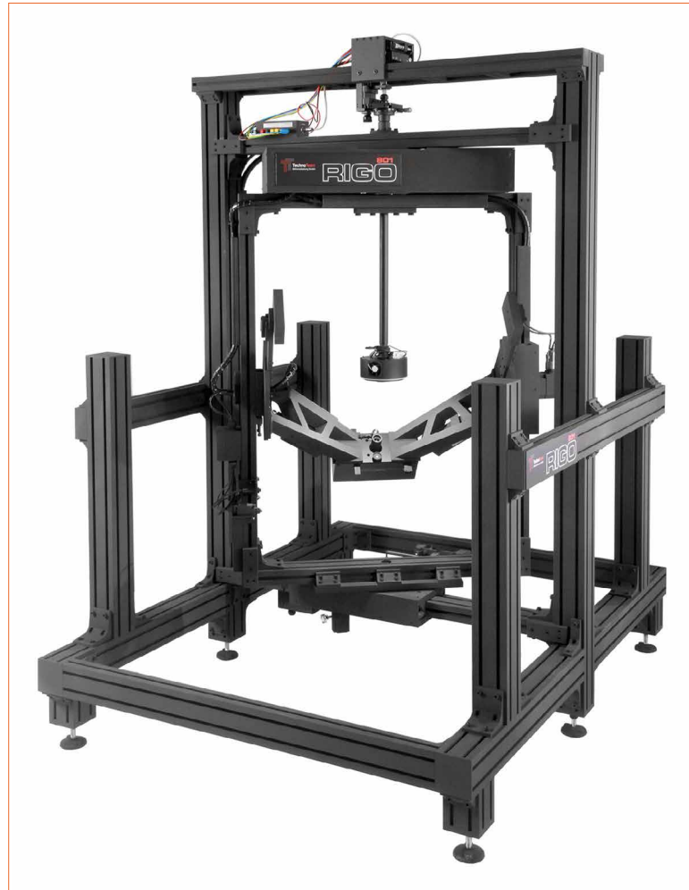
Figure 1: Conventional near field goniophotometer with two moving axes
