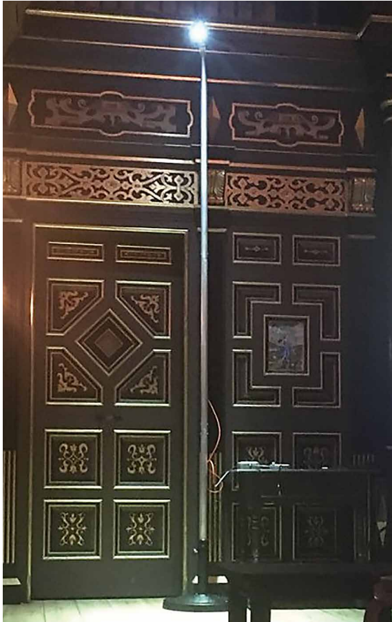
Figure 11: Street light demo with blue laser light transported several meters by fiber to a phosphor element at top with optic (Credit: Society of Light & Lighting)
