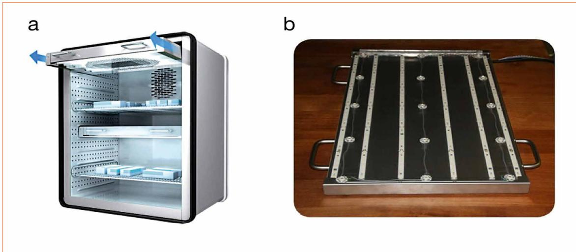
**Figure 6a&b:** Constant climate chamber (a) for photostability tests of the company Binder showing a flexible positionable light module traditionally equipped with fluorescent lamp. The prototype (b) equipped with 15 UVA LEDs uniformly distributed (0.9 W) and 8 cool white LEDs strips horizontally and vertically distributed (6300 lm)
