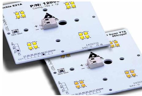
**Adura LED Solutions new MC12096 modules are based on CSP LED package from both Nichia and Seoul Semiconductor**
