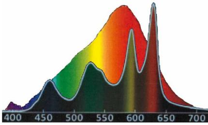
Comparison between a multi-chip LED solution and the Allix Xenoled technology that has a smooth continuous spectrum like the sun, while the multichip solution also shows no significant blue spike, but it has a poor SPD
