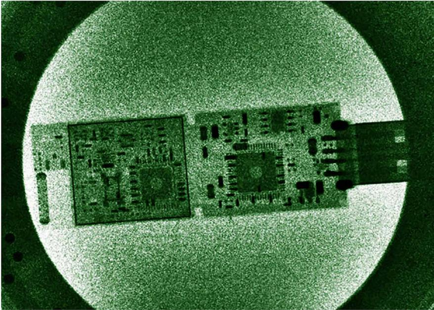
**Extreme Light Laboratory | University of Nebraska-Lincoln** - Using a laser focused to the brightest intensity yet recorded, physicists at the Extreme Light Laboratory produced unique X-ray pulses with greater energy than their conventional counterparts. The team demonstrated these X-rays by imaging the circuitry of a USB drive
