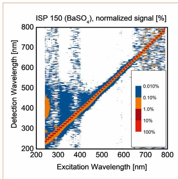
Figure 4 (left): Normalized spectra of discrete laser excitation at different wavelengths in a BaSO<sub>4</sub> ISP
