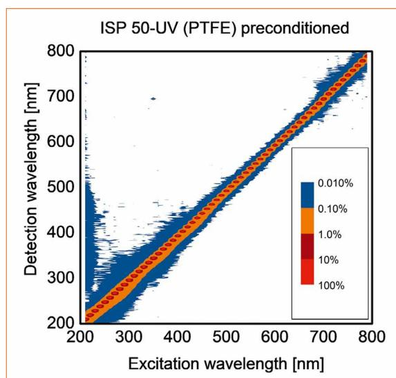
**Figure 9 (right):** Both measurements were acquired with calibrated equipment. The additional “blue” signal which is visible in both spectra is caused by the housing of the LED
