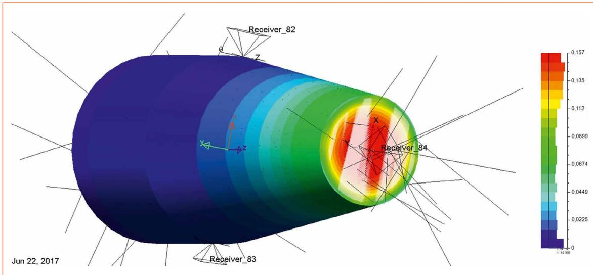
**Figure 3:** Optical simulation of light coupling from a fiber bundle into the glass condensing cone of the endoscope. The receivers placed on the surface of the condensing cone show the regions in which most of the radiation losses occur (green color)
