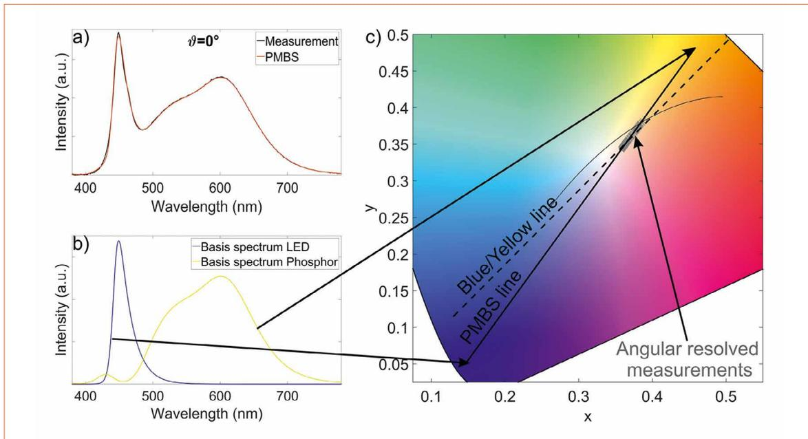
**Figures 3a-c:** PMBS: Reconstructed spectrum (a) at main radiance direction ( $\theta = 0^\circ$ ), global basis spectra (b) after spectral separation, and their associated mixing line in the chromaticity diagram (c)
