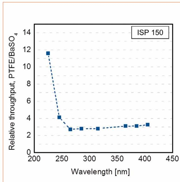
Figure 2 (left): Typical reflectivity of BaSO<sub>4</sub> and PTFE materials in the UV spectral range
