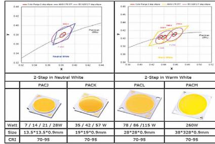
ProLight Opto's new CoB G-II Series LEDs offer high performance while providing high CRI and narrow 2-step MacAdam ellipse binning
