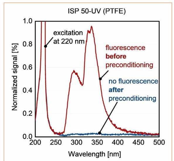
**Figure 8 (left):** Fluorescence matrix of the same PTFE ISP as in figure 6 after preconditioning. Fluorescence is efficiently suppressed to a level well below 0.1% for the entire UV spectral range
