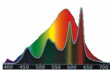
Comparison between a multi-chip LED solution and the Allix Xenoled technology that has a smooth continuous spectrum like the sun, while the multichip solution also shows no significant blue spike, but it has a poor SPD
