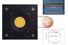
LES comparison for YUJILEDS' High Density High CRI CoB. CRI test result of 5600 K CoB sample (top inset). Burn-in test and lifetime calculation result of High Density High Power CoB (bottom inset)
