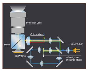
control is enabled, without the need for large arrays of LEDs. By combining laser light and a liquid crystal or micro mirror device in a small form factor, efficient package, automotive and specialty lighting applications may benefit.
