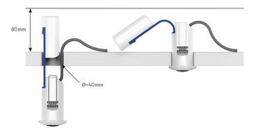
Tridonic's new EM ready2apply emergency lighting system is based on lithium-iron phosphate battery technology and it is easy to install
