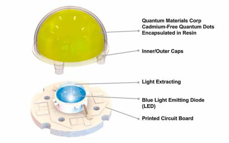
The DUT for the reliability test is a remote QD mid power LED consisting of the components shown on the image  $% \left( \mathcal{A}^{\prime}\right) =\left( \mathcal{A}^{\prime}\right) \left( \mathcal{A}^{\prime}\right)$
