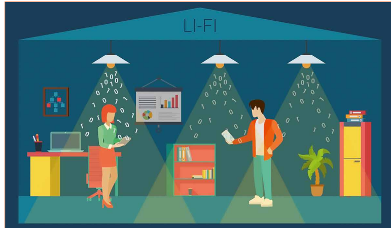
Figure 2: Exemplary data transmission in an open office space via LED light bulbs
