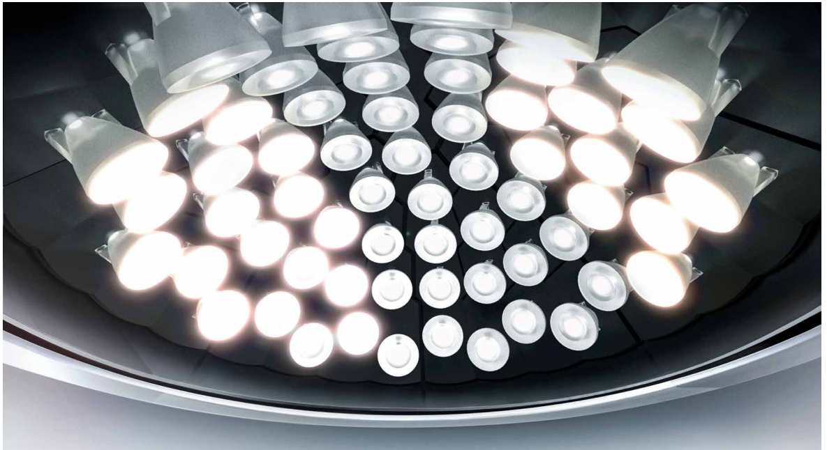
Figure 2: Detail of the “Omnipoint” demonstrator: Each LED with its own lens shines into a different angle and therefore illuminates a different area in the room
