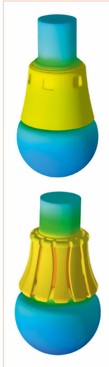
Figures 6&7: Simulation models of two different LED replacement lamp designs
