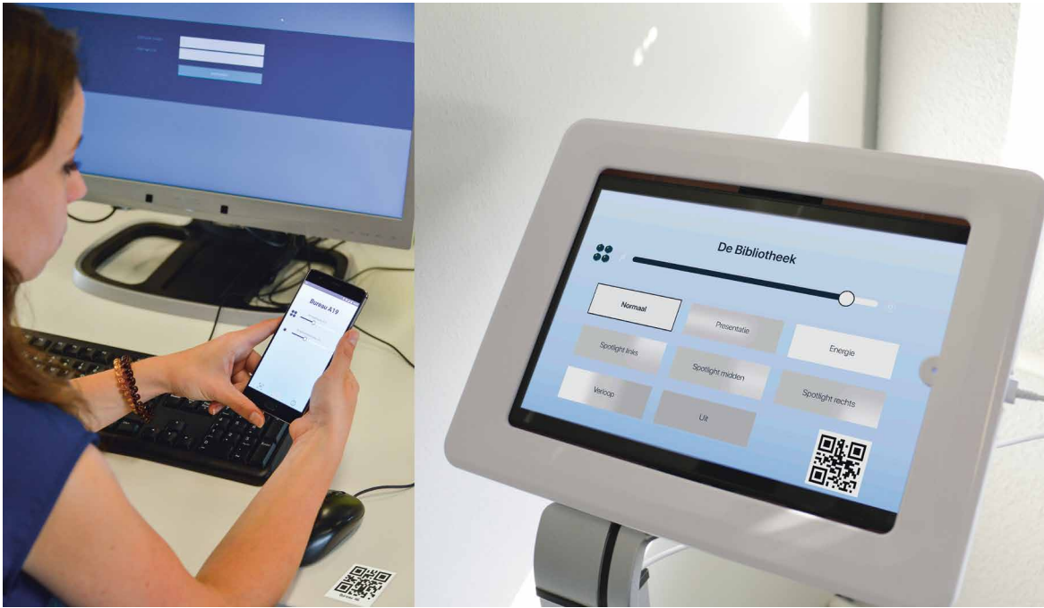
Figure 3: User apps: (left) the phone app, and (right) the room control tablet in a meeting room
