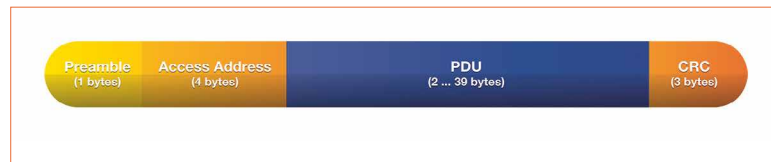
Figure 2: Basic BT message communication format
