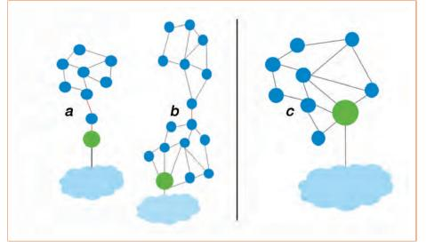
Figure 3: A bad solution for the implementation of the sink node (a) and a bad solution for the mesh design (b) versus a better solution (c) for both
