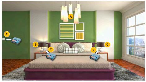
Figure 3: Smart home upgrade in a bedroom with 3 luminaires and 3 on/off switches
