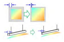
Figure 4: Reduction of blindfold for edge lit solutions (Top), reduction of size of pendant solutions (Bottom)
