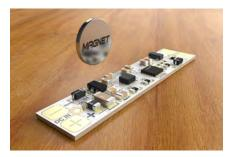
Cezos' new magnet switch, L475T, with its ultra-low-power high-performance three-axis magnetic sensor offers many useful features for its applications like inside cabinet LED lighting
