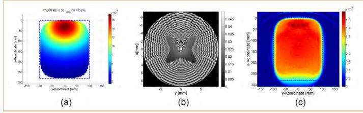
Figure 2: a) Simulated irradiance distribution within the oval shaped target area without FF-MOE. b) Calculated structure of the FF-MOE with a maximal height of 50um. c) Simulated irradiance distribution within the oval shaped target area with FF-MOE
