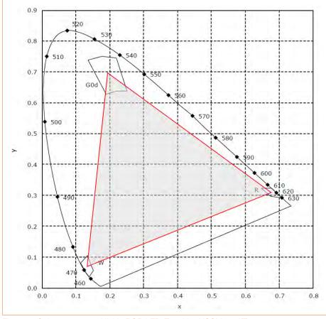
Figure 1: Color gamut of a Nichia RGB LED (Part No. NSSM240AT)
