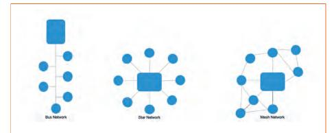
Figure 1: Schematic examples of a linear network, a star network and a mesh network structure
