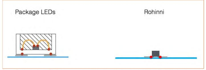
Figure 2: Traditional packaged LEDs (left) are connected at multiple points, while direct-placed mini/micro LEDs (right), with only two points of connection, are much less prone to failure
