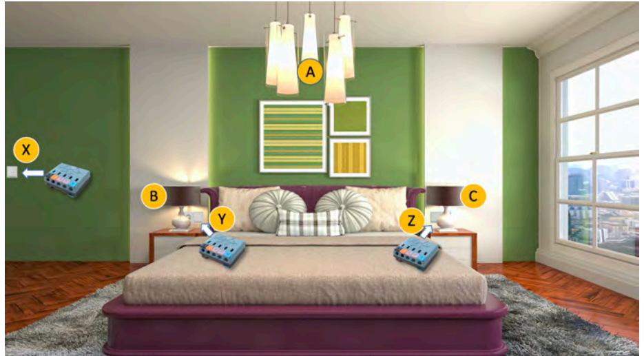
Figure 3: Smart home upgrade in a bedroom with 3 luminaires and 3 on/off switches
