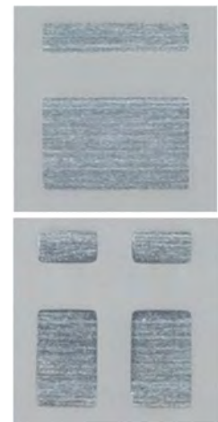
Figure 3: Footprints of 3030 mid-power packages. Standard package (Top), 2-in-1 package (Bottom)
