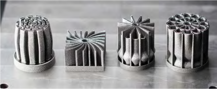
Figure 6: 3D Printing one-piece heat sinks for lighting applications
