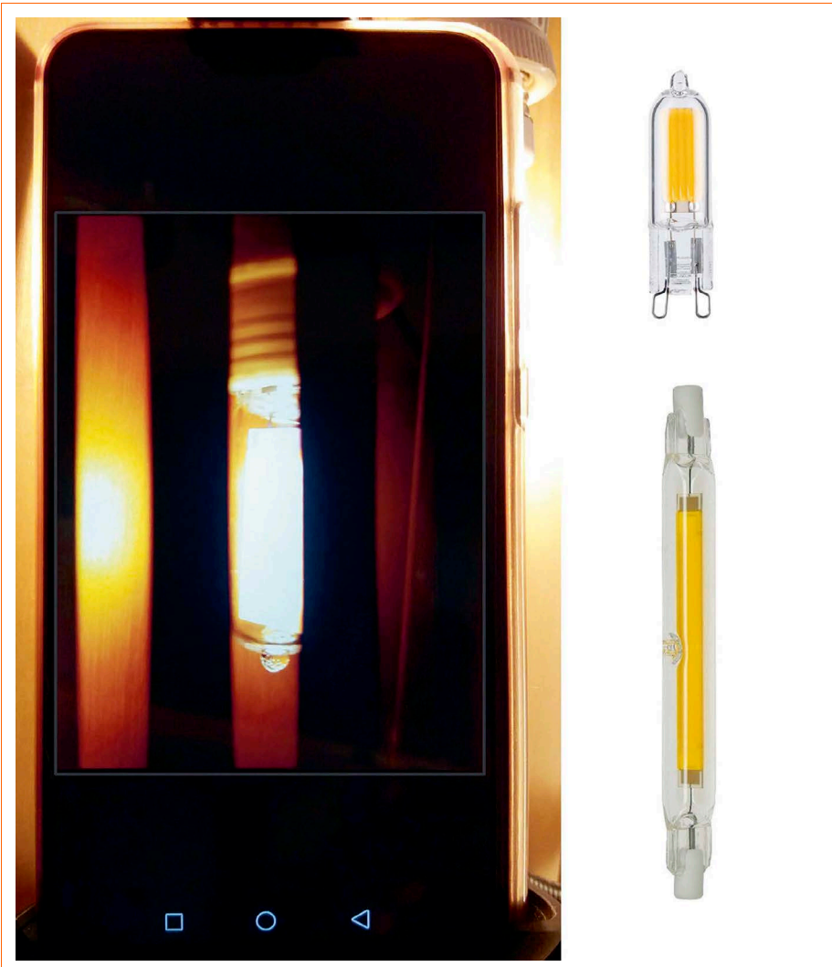
Figure 8: Self-help via smartphone to make network-dependent flicker visible
