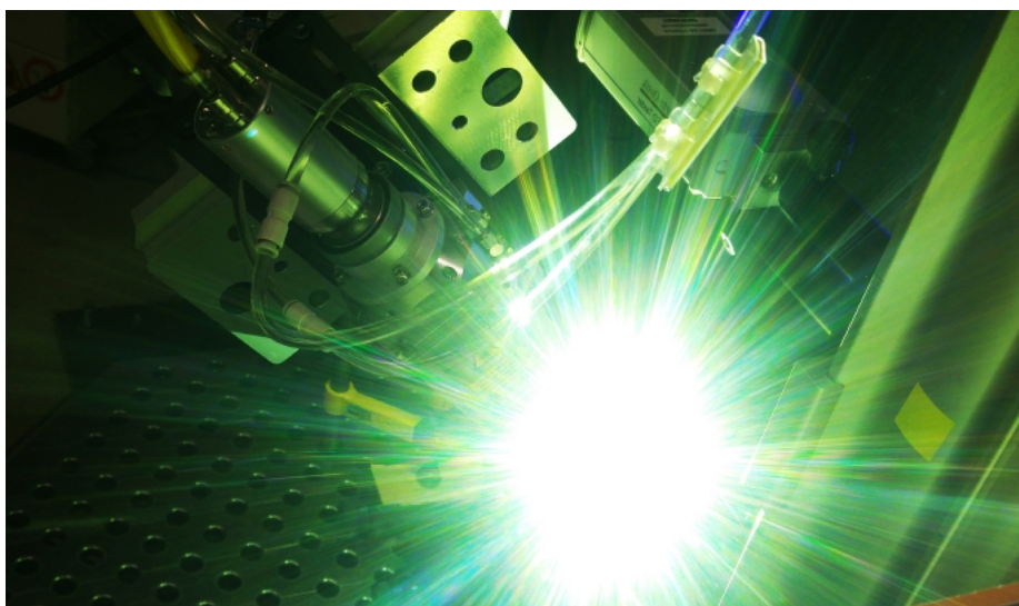
Figure 4: The blue laser light is for the most part absorbed by this phosphor converter and then re-emitted at longer wavelengths. The result is a white broadband light spectrum. ©Laserline
