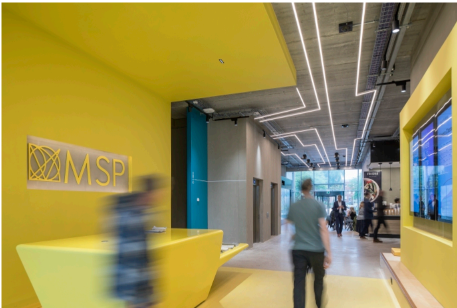
Figure 2: Bright Building Manchester Science Park © BDP, Nick Caville. The design satisfied many of the BDP Circular Economy principles. The main ones were "Building in Layers" and "Design for Disassembly" as all the lighting used surface mounting techniques avoiding recessing and integration. Secondary factors were "Designing out Waste" as the design was highly optimized and "Design for Adaptability" – the surface mounted principle allows for spaces to be easily reconfigured by swapping out luminaires to create new environments when and as needed.
