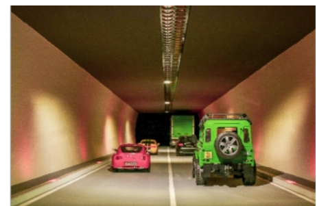
Figure 14: Counter-beam (left) and pro-beam (right) lighting in the dynamic tunnel model Bartenbach.
