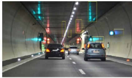
Figure 4: Exemplary situation in the tunnel; luminance levels and information in the visual field.
