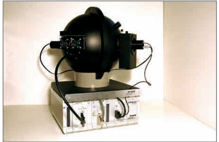
Figure 6: The TERALED extension for the T3ster thermal transient tester provides high accuracy experimental radiometric and thermal data of LEDs
