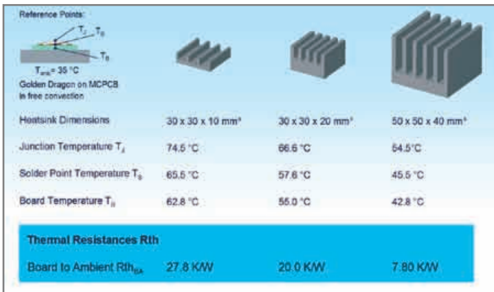
Figure 15: Thermal Resistance RthBA of different heat sinks
