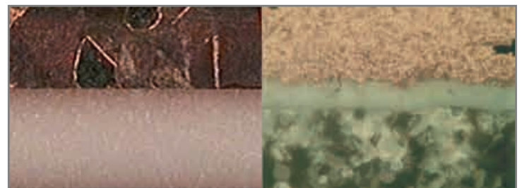
Figure 3: Interfaces on both alumina (left) and aluminiumnitride (right)
