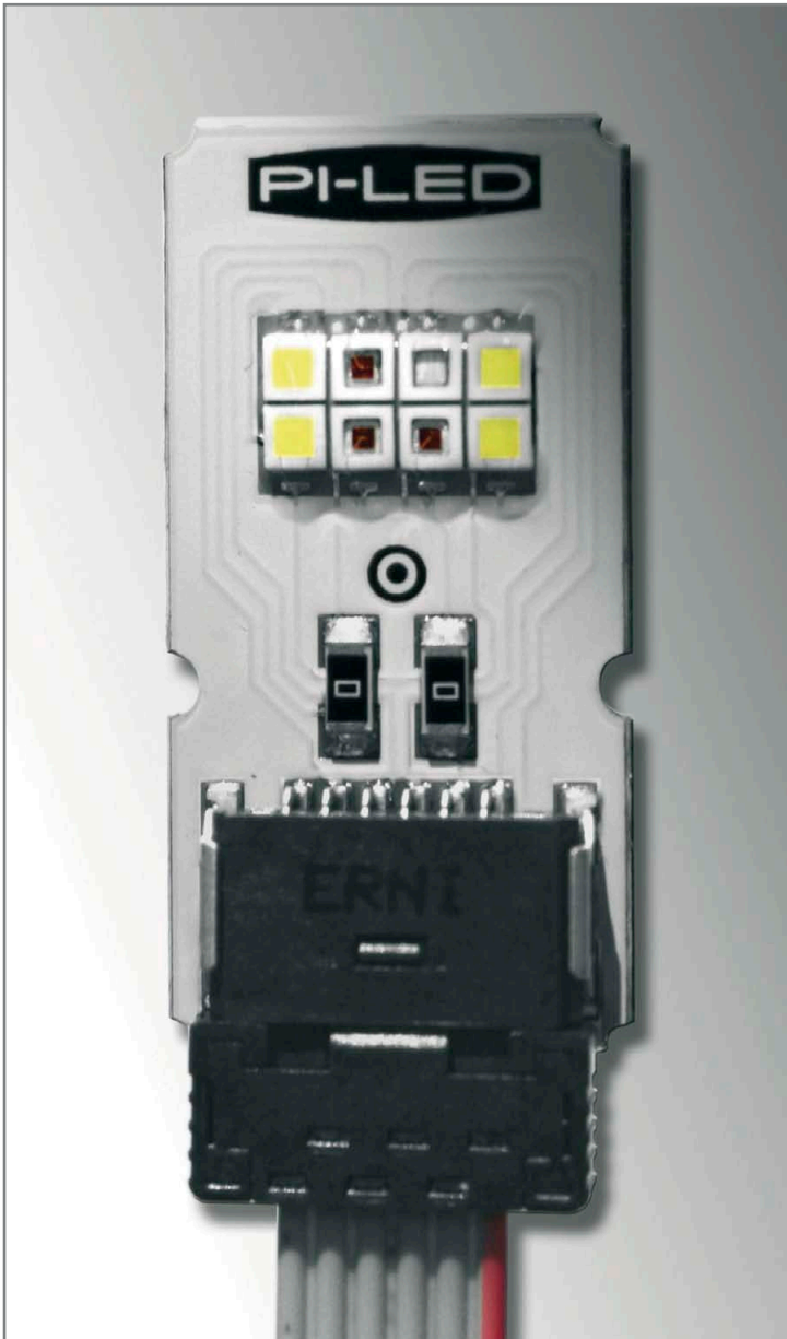
Figure 7: PI-LED module with four phosphor LED's, three red LED's and one blue LED
