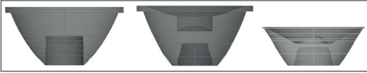
Figure 10: Schematic views of two commonly available Luxeon collimators (left and center) and the LPI UFO (right). All three designs have similar exit apertures and collimation angles. The two designs on the left have plastic volumes of approximately 1500 and 1300 mm 3 respectively, while the LPI UFO (right) has a volume of about 500 mm 3 .
