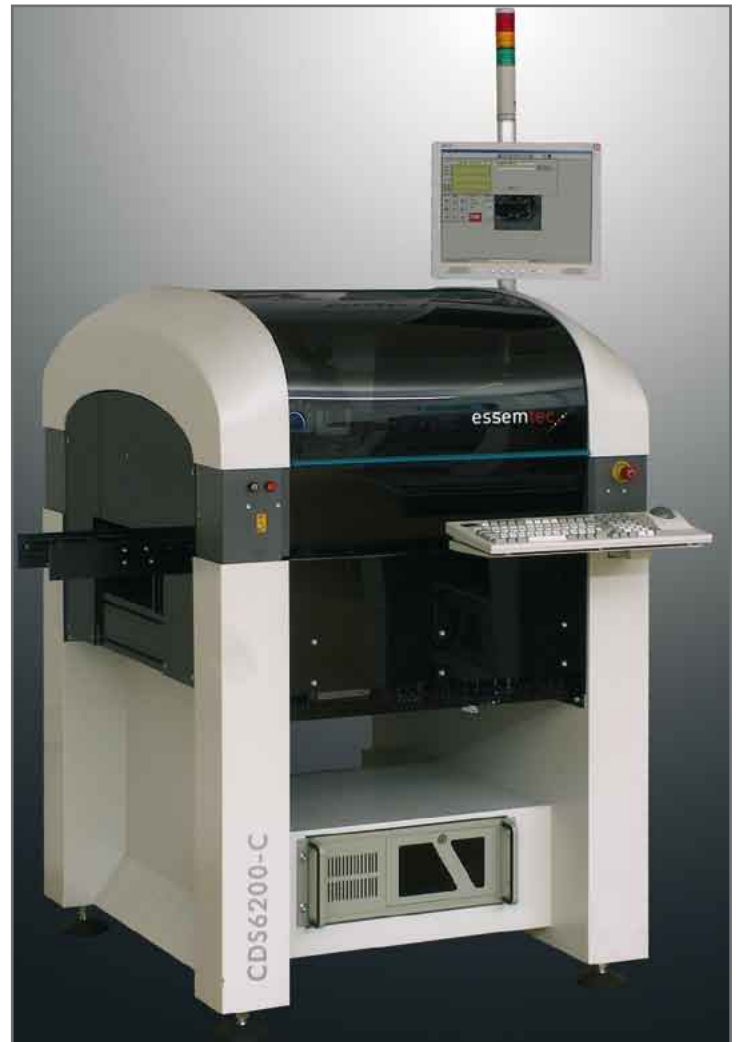
Figure 5: An automatic dispensing system with high accuracy and versatile flexibility
