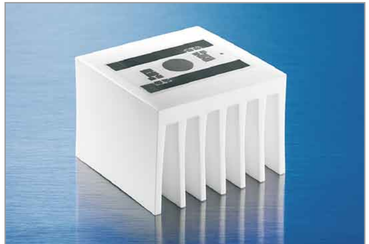
Figure 3: First serial production of optimized CeramCool geometry for 4W cooling. With Rubalit the total thermal resistance R_{tt} of the assembly is at least 13% better than aluminum. Using Alunit it is more than 31% better.
