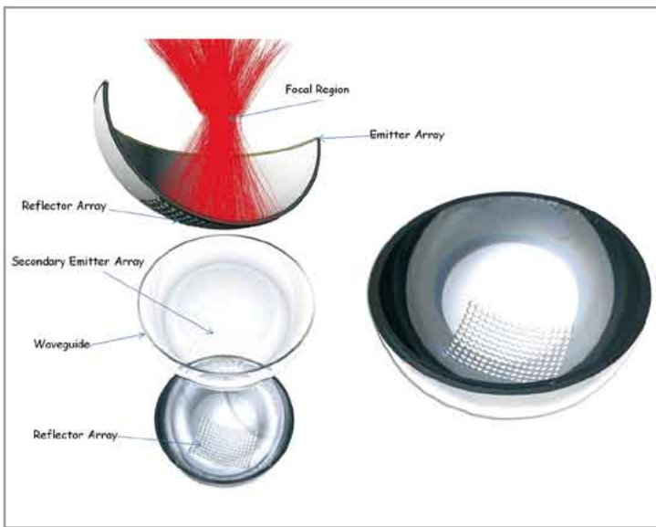
Figure 5: An example of concave illuminator design
