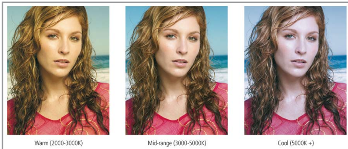
Figure 3: Other than most light sources, LEDs can be manufactured in a wide range of CCT from 2200K to over 11500K, making LEDs the first choice for different applications from residential lighting to medical applications
