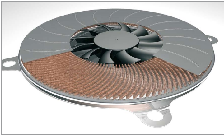
Figure 11: A circular system consisting of a contra-spiral manifold with VTIPs and ventilation
