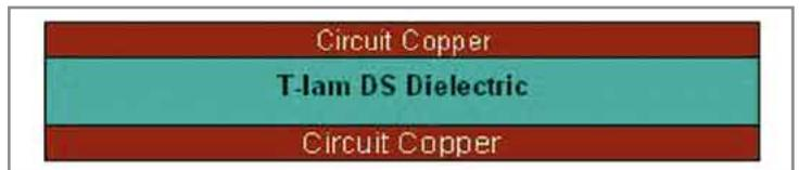
Figure 3: T-lam DS Substrate Illustration.
