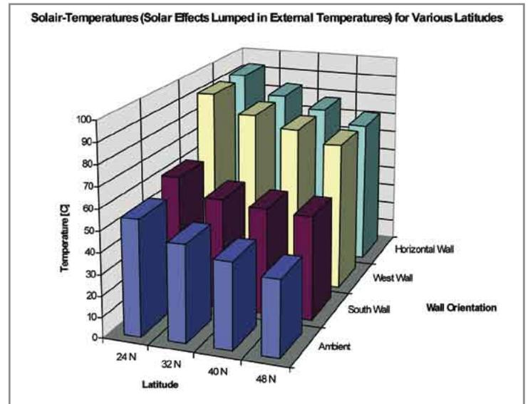
Figure 2: Typical Sol-Air temperatures for various latitudes.
