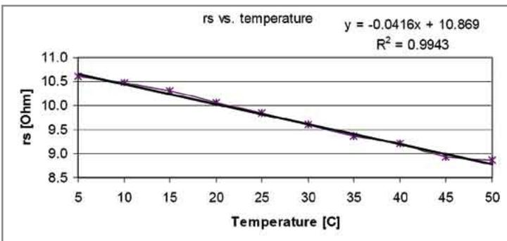
Figure 12: Temperature dependence of model parameter  $r_s$ .
