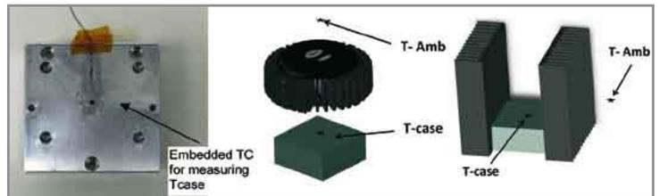
Figure 6: Thermocouple locations.
