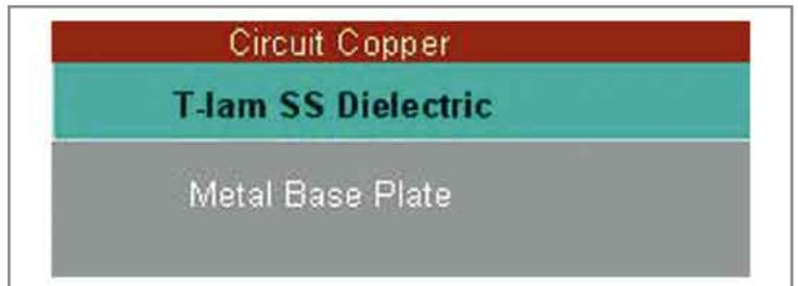
Figure 2: T-lam SS Construction.
