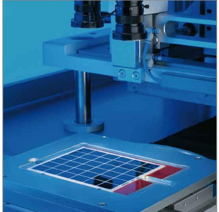
Figure 11: In a final step before the final inspection metallization pads and electrical circuit tracks are applied.
