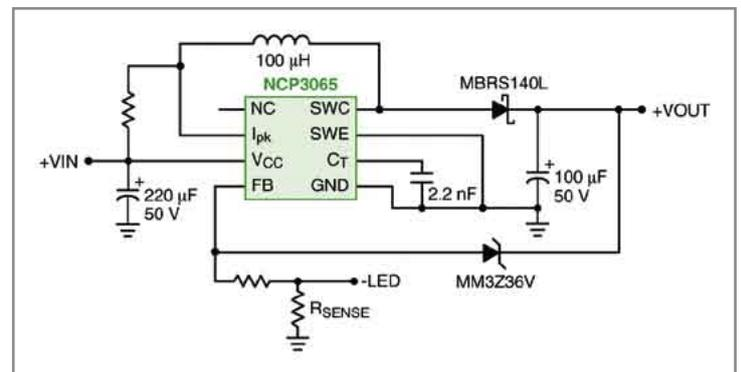
Figure 3: Typical schematic of a Boost Converter.
