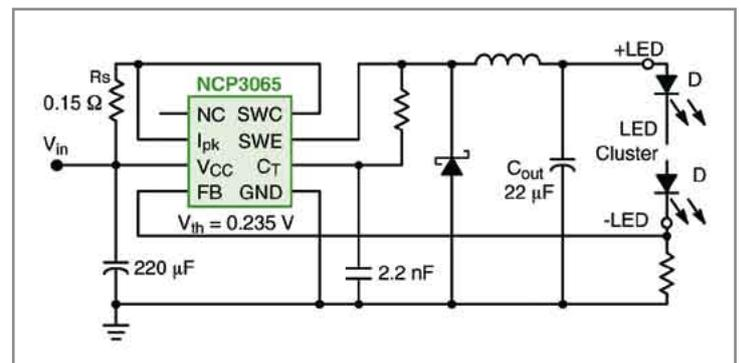
Figure 2: Typical schematic of a Buck Converter.
