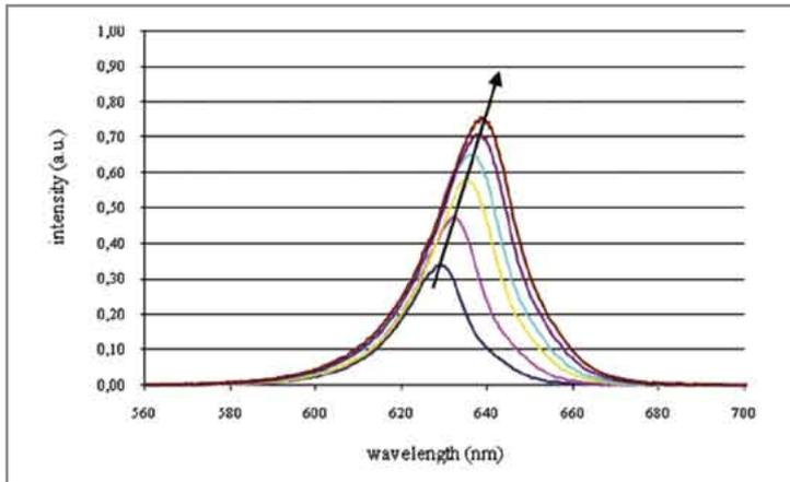
Figure 1: Wavelengthshift with rising LED junction temperature  $T_j$ .
