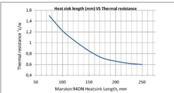
Figure 11: Rs-a vs. heat sink length (Source: Marston 94DN Datasheet).
