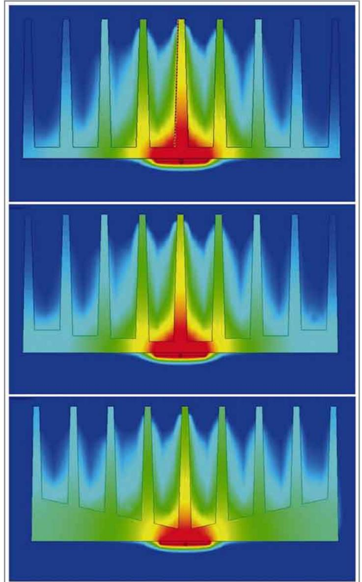
Figure 4: Product development can be supported by a simulation process allowing customer specific thermal optimization (Source: Altair Engineering).
