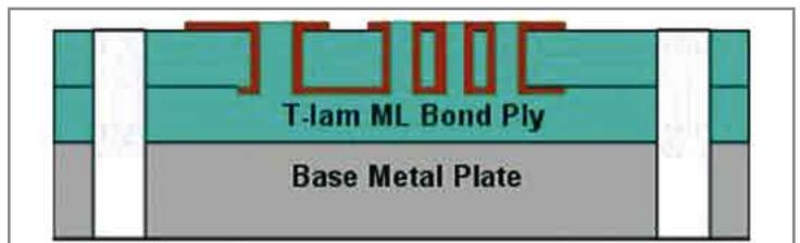
Figure 4: T-lam ML Circuit Illustration.
