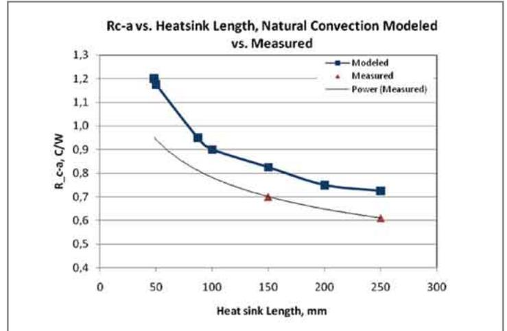
Figure 12: Modeled and measured Rc-a vs. heat sink length.
