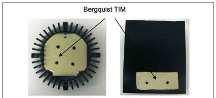
Figure 8: Bergquist GP2500S20 installed on heat sinks.
