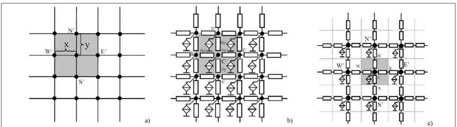
Figure 3: Models in 2D a) Finite differences grid b) Finite differences model c) Vector SUNRED model. - The description of the successive node reduction method can be found in earlier publications such as [3] and [10].
