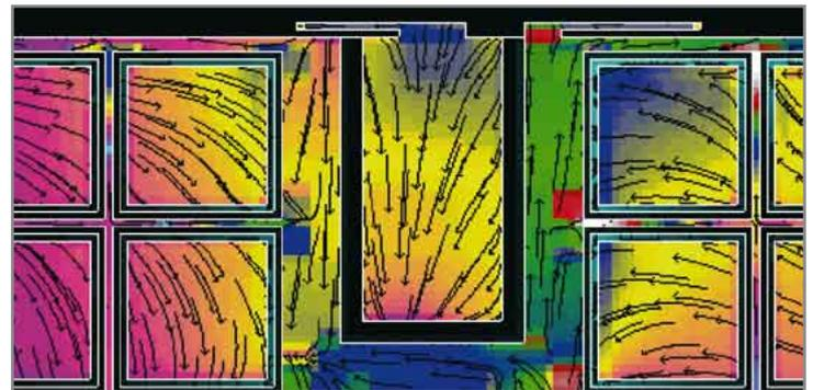
Figure 10: Electrical current density distribution in the ITO layer when a medium sized shunting grid was assumed.
