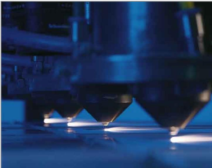
Figure 7: Laser treatment permits a wide range of thicknesses, the tightest tolerances and short turnaround times. The process is economical for both small and large quantities.
