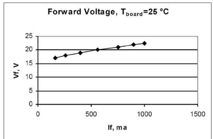
Figure 2: Diode forward voltage as a function of forward current, based on data in [1].
