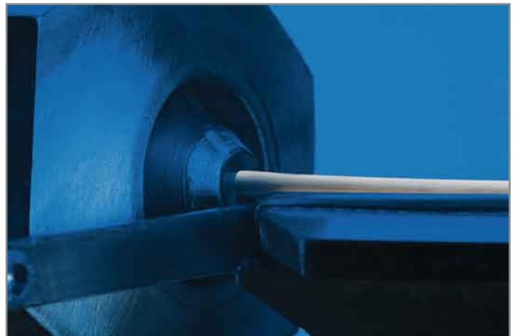
Figure 9: Extrusion is an economically viable process for mass production of rotationally symmetrical components such as rods and pipes. Lengths from 3mm up to 400mm are possible. The diameters for rods range from 0.5mm to 20mm, and in pipes diameters up to 40mm can be produced.
