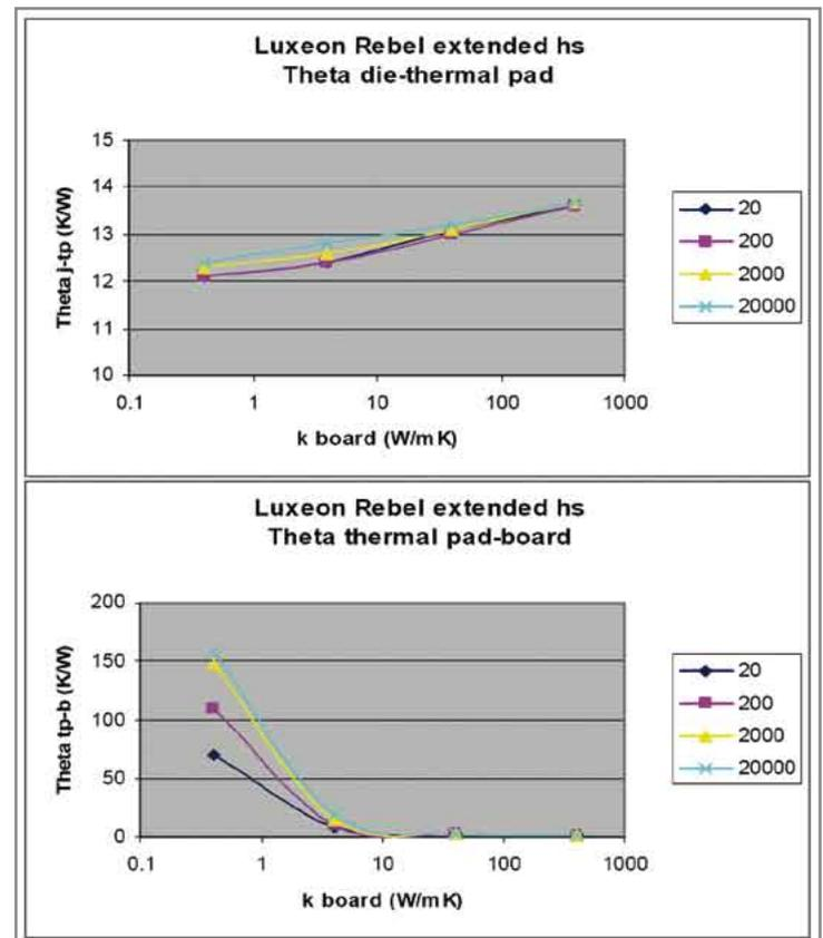
Figure 7: Graphs demonstrating the drawbacks of the series-resistance approach with  $h$  between 20 and 20000 W/m<sup>2</sup>K as parameter. Top: Resistance die-thermal pad, Bottom: Resistance thermal pad-board.
