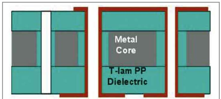
Figure 6: T-lam ML Metal Core Illustration.
