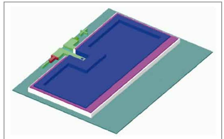
Figure 5: Simulation model of the OLED seen in Figure 2.
