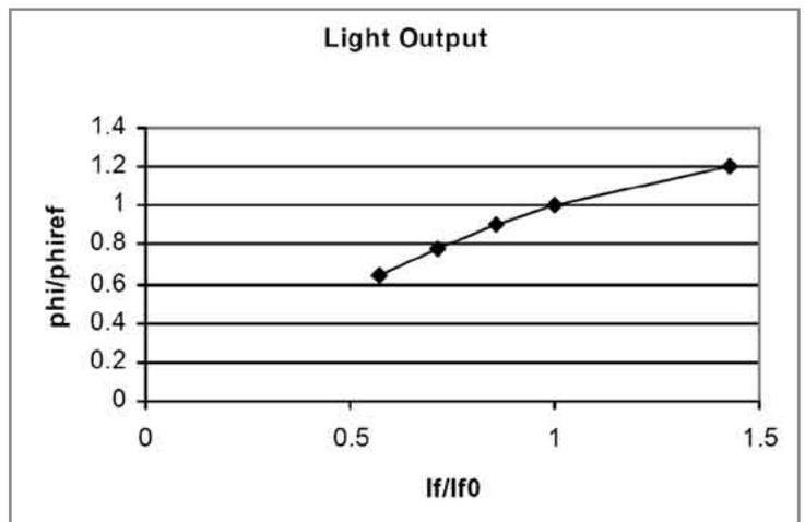
Figure 4: Relative light output as a function of current ratio.
