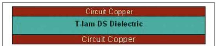
Figure 3: T-lam DS Substrate Illustration.
