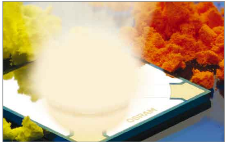
A new converter mix that OSRAM is currently testing in its development laboratory provides a pleasant warm white light.
