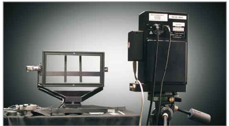
Figure 6: Measurement of large LED luminaires. By directly measuring large light sources from within the near-field, a combination of a two-axis goniometer and imaging colorimeter can obtain detailed performance measurement in a compact laboratory space.
