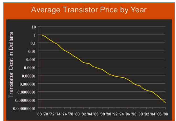
Figure 1: The historical trend for the average transistor price shows the continuous cost reductions achieved by the Semiconductor Industry [3]. Of the 4,000,000x cost reduction between 1975 and 2008, approximately 500x is due to manufacturing efficiency improvements.
