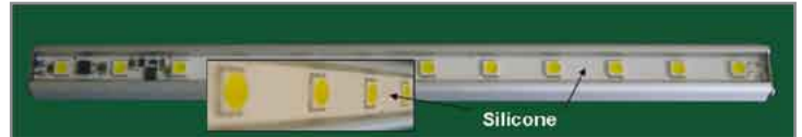
Figure 5: LED light bar sealed using a 40 Shore A optically clear silicone encapsulant.
