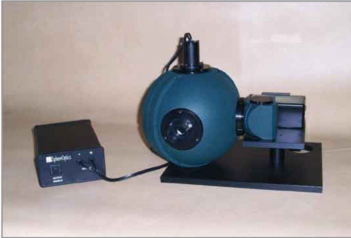
Figure 5: High Power LEDs measured with two Integrating Spheres.
