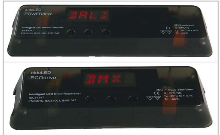
Figure 4: Whether in DMX, DALI or DALI Color it is clear that LED lighting electronics are evolving rapidly to enhance lighting networks by providing local feedback to the controller, by gracefully adjusting fixture power settings to stay within operating (temperature) limits or by adjusting the mix of separate colors based on local temperature or color feedback.
