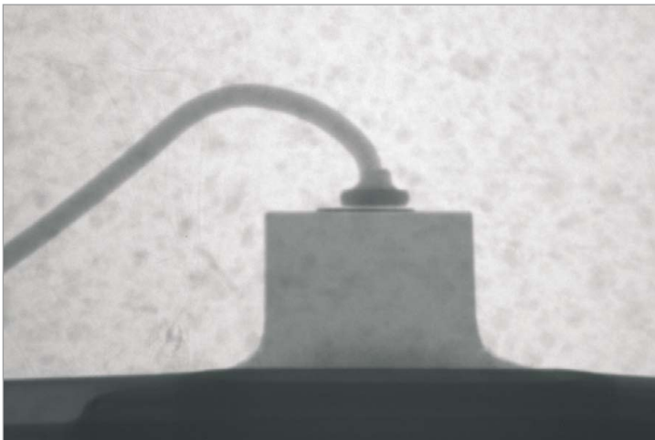
Figure 6: Detachment of bond wire from the chip – x-ray microscopy.
