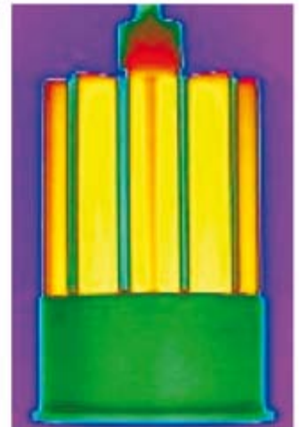
Figure 3: An LED-based spotlight with around finned heat sink. Visible and IR views
