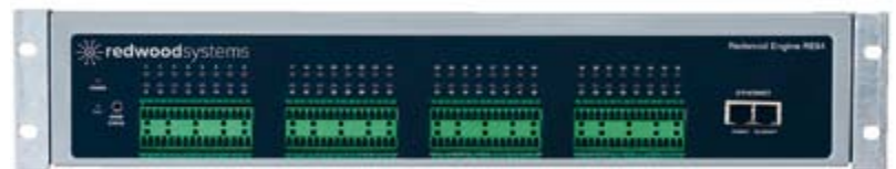
Figure 1: Centralized LED Driver and Control Engine
