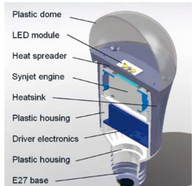
Figure 6: Cross section of the prototype bulb
