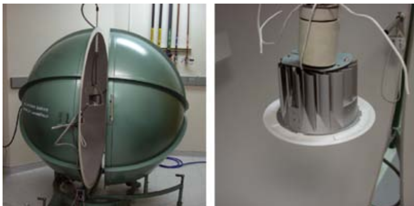
Figure 8: (a) 1.5 meter integrating sphere. (b) Mounted down light in sphere
