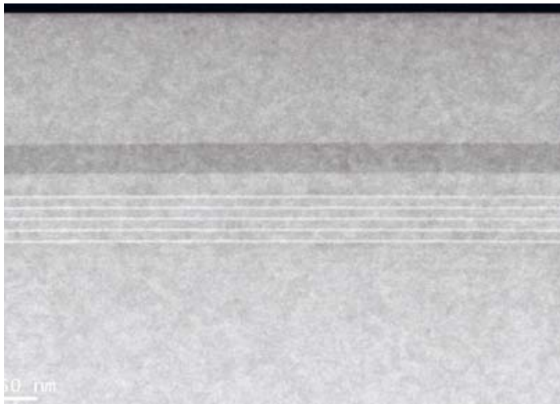
Figure 5: Cross section TEM of the active region
