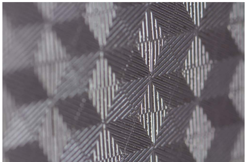
Figure 6: PMMA is Evonik's established product for several (lighting) applications, while SAVOSIL™ is the new high-end material predestined for LED and PV applications. Currently under development is a technology of SAVOSIL to create a microstructure on panels. The microstructure was printed onto a PMMA sheet.
