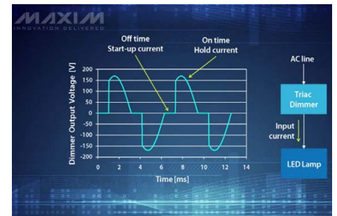
Input current shaping of the MAX16841 satisfies the requirements of triac dimmers on start-up current and hold current to avoid flicker at low dimming values
