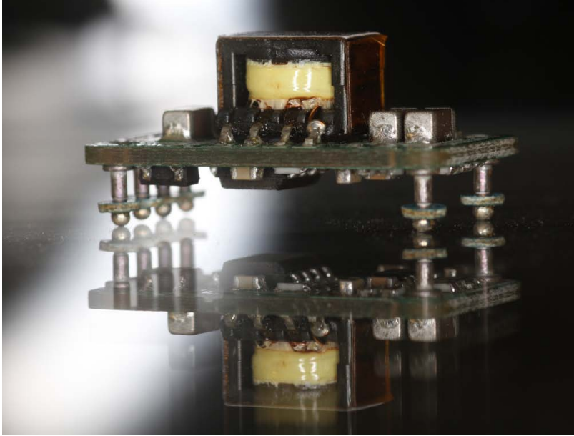
Figure 14: Recom also provided insight into driver details, showing the assembled PCB
