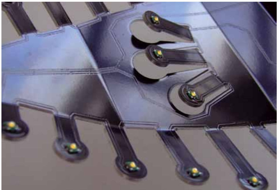
Close-up of a formable thermal LED PCB solution from DK Thermal Solutions
