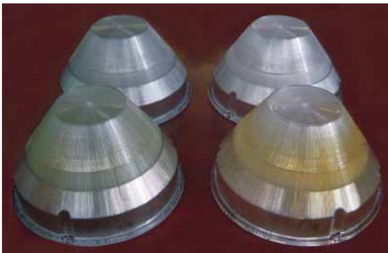
Figure 3: Yellowing due to UV exposure is one major problem in outdoor applications. Improved PCs retain their gloss and color stability up to 5 times longer than standards PCs
