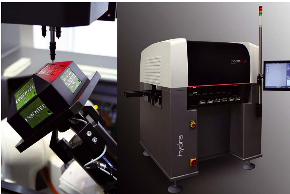
Essemtec's Hydra dispense and placement system allows 3D placement of electronic components, including LEDs
