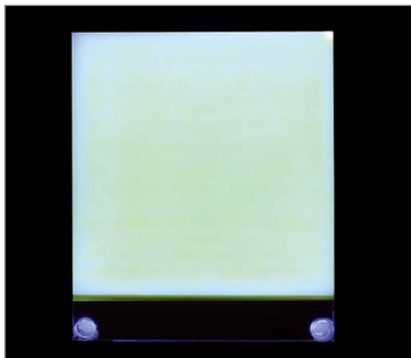
Figure 8: The PRP-module output light uniformity – (a) top view, (b) and (c) lateral and longitudinal intensity distributions, respectively
