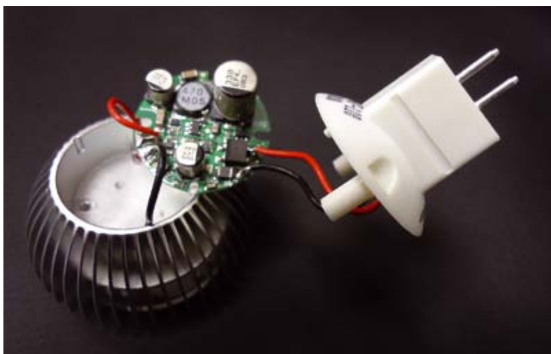
Figure 1: Typical electronics that is used to drive DC LEDs, in this case from an MR16 lamp
