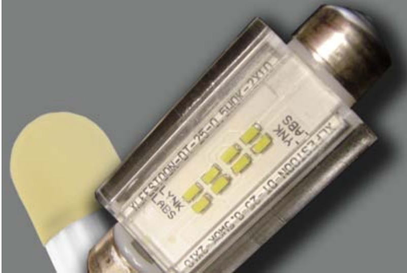
Figure 3: Examples par excellence for driverless lamps are festoons or bi-pin capsules, due to a limited space for the electronics
