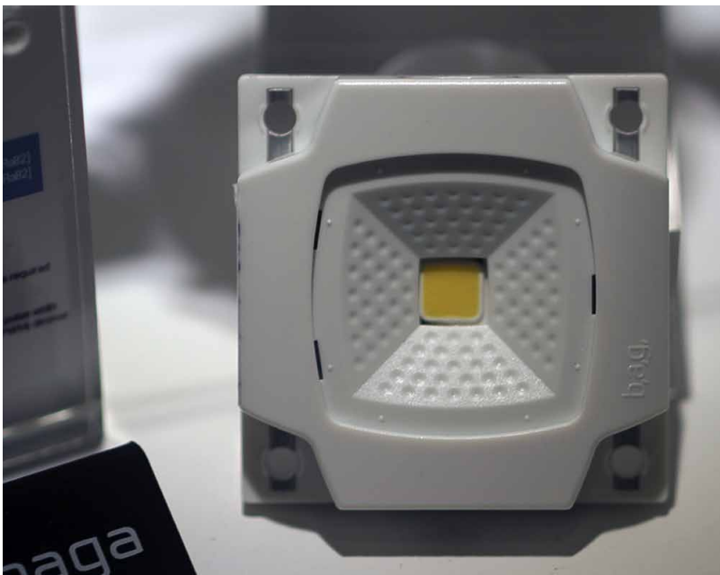
Figure 12: b,a,g, presented one of the first Zhaga Book 7 compliant LED modules
