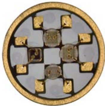
Figure 8: COB technology in detail showing bonding wires and semiconductor placement
