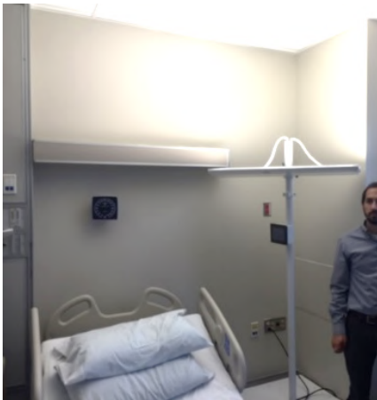
Figure 1: The experimental luminaire used to deliver the BWL (active) and DWL (inactive) interventions in participants' rooms.
