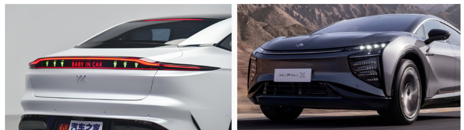
Figure 7: SAIC's IM L7 rear applique display (left) and HiPhi X Intelligent Signal Display (right).
