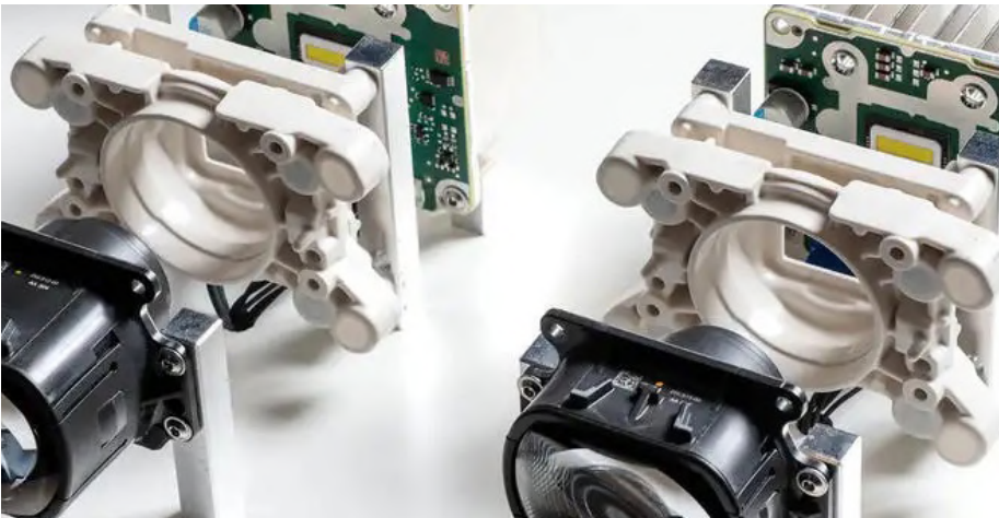
HD Matrix LED Headlights with 16,384 micro-LEDs per LED array. Photo credit: Porsche.
