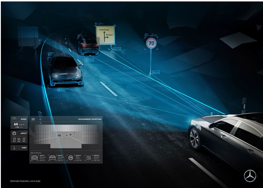
Powerful computers evaluate the data and give the headlights commands for the best possible adjustment of light distribution in all situations. To avoid glare as much as possible, the light is dimmed for oncoming or preceding vehicles, other road users, and traffic signs. Photo credit: Daimler AG
