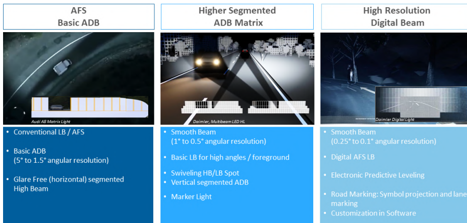
Figure 1: Adaptive Driving Beam pattern granularity and key application benefits. From AFS/ADB to high resolution digital beam.
