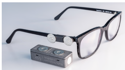
The light-dosimeter (lido) is a mobile measurement device used to investigate the non-visual responses to light.
