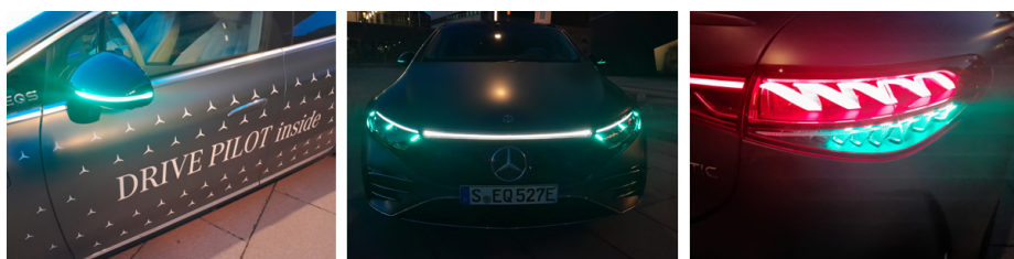
Figure 5: Mercedes EQS drive pilot concept featuring cyan marker lights for automated driving mode. Function demonstrated in headlamp, rearlamp and side mirrors (ISAL 2023).
