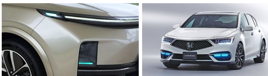
Figure 4: Li Auto 'L9' with cyan ADS marker lights (left) and Honda Legend hybrid; world's first certified L3 car with cyan front marker lights (right).
