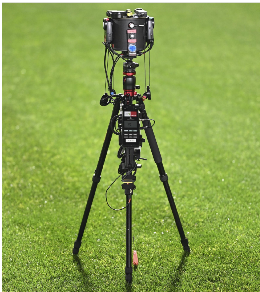
Figure 6: The horizontal and vertical illuminance measurement system ( EhEv Tripod Mount ), developed by Dr. Perez , met all requirements during the FIFA Floodlights Test Event in Rabat and was documented in the official FIFA test event report.
