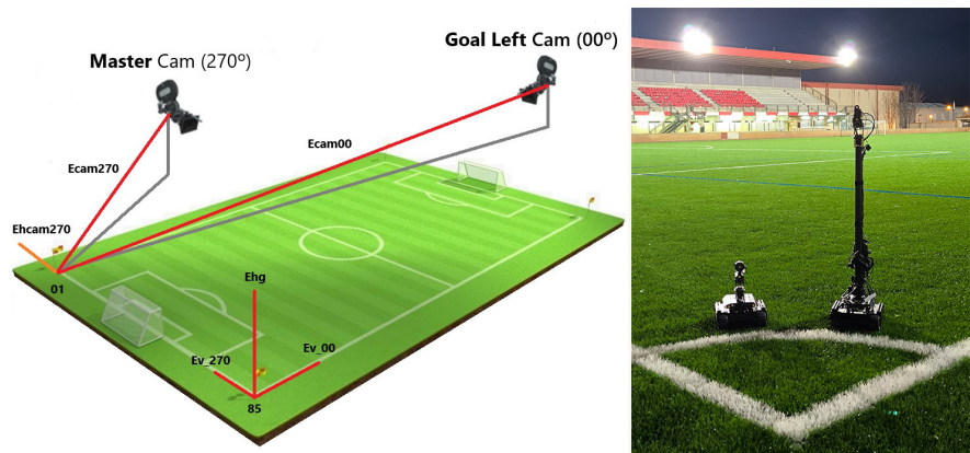
Figure 1: One of the most demanding standards is the one from "LaLiga" in Spain, a private standard, where E_{cam} shall be taken against (normal to) four (4) reference cameras all over the pitch.
