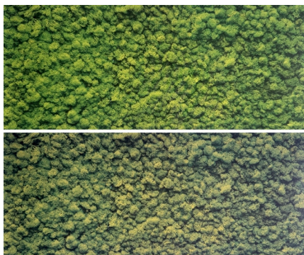
Figure 3: 3,500 K light source on the Planckian locus (top) versus a 3,500 K tunable white source with a deviation of >10 SDCM from the Planckian locus (bottom). © Lumitech. Real photographs; no image editing or AI used.
