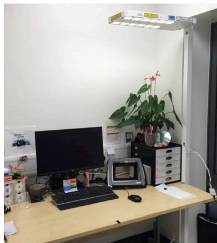
Figure 8: Floor lamp providing white light at the desk, modified with LEDs emitting ultra-low levels of UVB.
